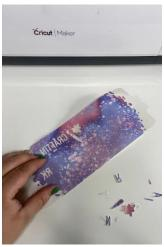
After completing the design, insert the material into the machine and press the **Load** button. The design will be cut quickly. Once the cutting is done, unload the material and use a weeding tool to peel away any unwanted parts from the design.
